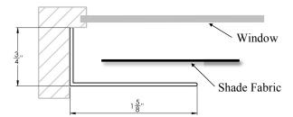
Attach the mounting channel with screws. Note: Top view shown.
