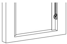
Side channels installed on the **inside** frame of the window
